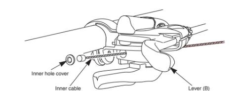
Connect the cable to the rear derailleur and, after taking up the initial slack in the cable, reattach to the rear derailleur as shown in the illustration.
