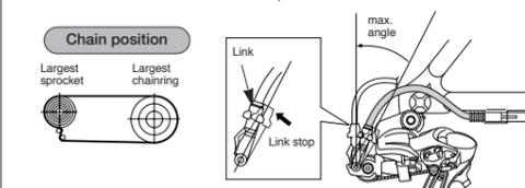
Connect the inner cable to the derailleur as shown in the illustration.
