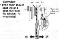
(2) Next with the chain on the 2nd gear, increase the inner cable tension ① while turning the crank arm forward. Stop turning the outer casing adjustment barrel just before the chain makes noise against the 3rd gear.
