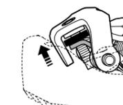
If the adjustment plate is at the strongest or the weakest position, do not turn the adjustment bolt any further.
