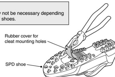
2. Remove the sockliner and position a cleat nut over the oval holes.
