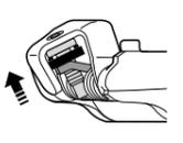
If the adjustment plate is at the strongest or the weakest position, do not turn the adjustment bolt any further.
