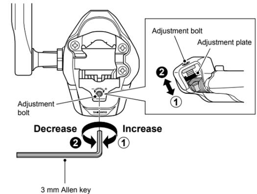
When the adjustment bolt is turned clockwise, the spring tension increases, and when it is turned counterclockwise, the spring tension decreases.
