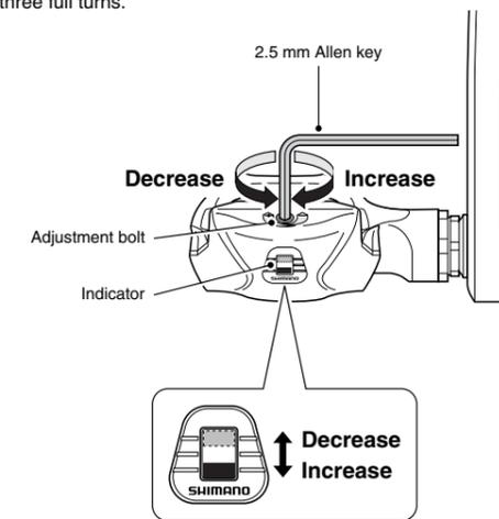
Do not turn the bolt past the point at which the indicator shows the maximum or minimum tension.
