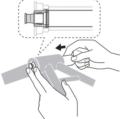
As shown in the illustration, hold down the flap with your fingers and push it in from the opposite side. (When pushed in, the flap opens.)
