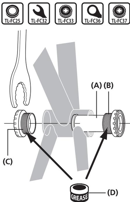
Grease the left and right hand adapters and use the Shimano original tool to install the right hand adapter of the bottom bracket, the inner cover and the left hand adapter of the bottom bracket.
