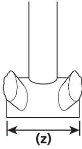
Check whether the width of the bottom bracket shell is 68mm or 73mm.
