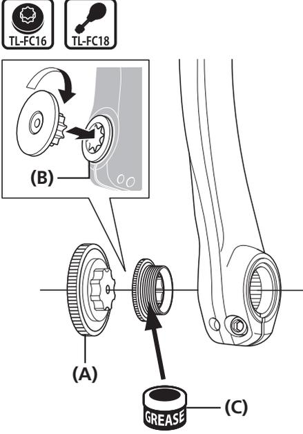
Use the Shimano original tool to tighten the cap.
