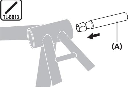
Insert the Shimano original tool into the bottom bracket.
