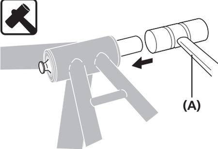
Tap the Shimano original tool with a plastic mallet until the end of the bottom bracket is ejected.
