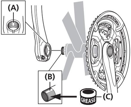
Set the wide groove area of the left crank arm into the axle of the right crank arm unit where the groove is wide.
