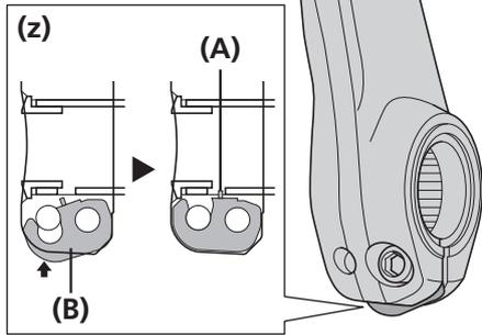
Push in the stopper plate and check that the plate pin is securely in place, and then tighten the bolt of the left crank arm.
