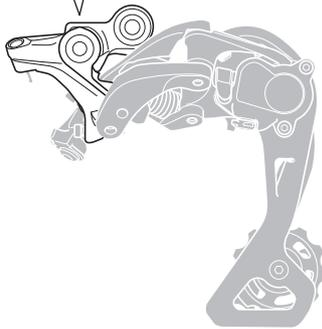
Remove the bracket axle.
