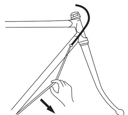
Remove the initial slack from the cable as shown in the illustration.
