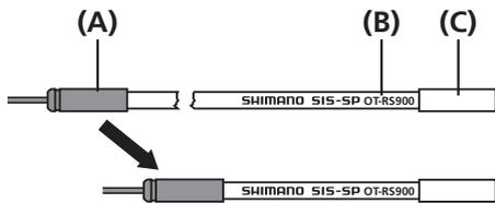
After cutting, attach the same cap with long tongue to the end.
