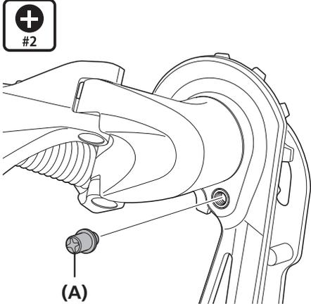
Remove the plate stopper pin.
