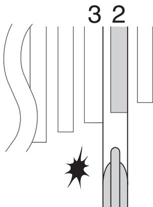
The best setting is when the shifting lever is operated just enough to close the lever gap and the chain touches the 3rd sprocket counting from the smallest sprocket and makes noise.
