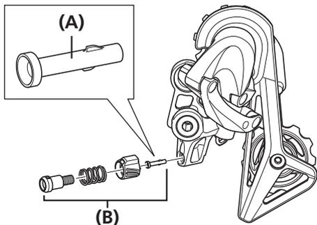
Remove the cable adjustment barrel and then remove the cover with tongue.
