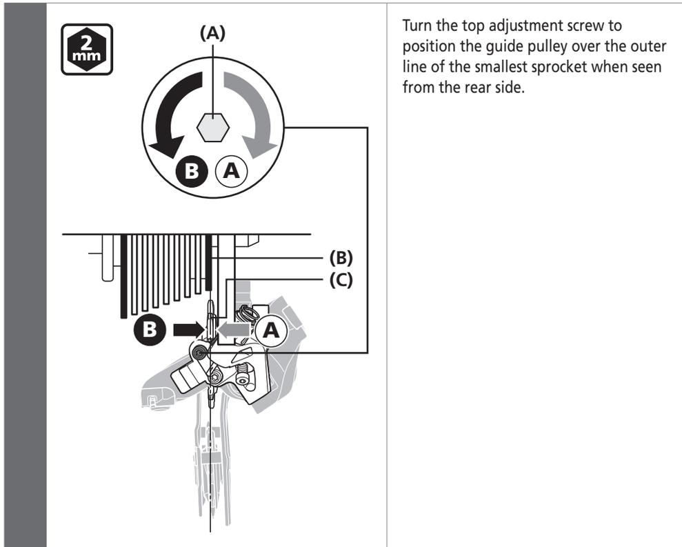
Turn the top adjustment screw to position the guide pulley over the outer line of the smallest sprocket when seen from the rear side.
