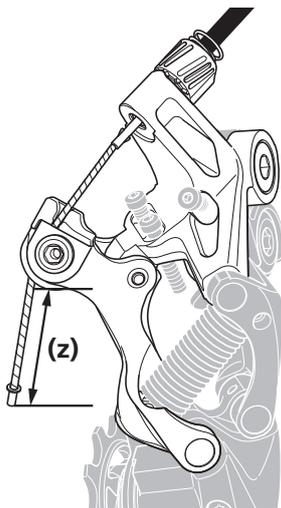
Set the inner cable so that the margin is approximately 30mm or less.
