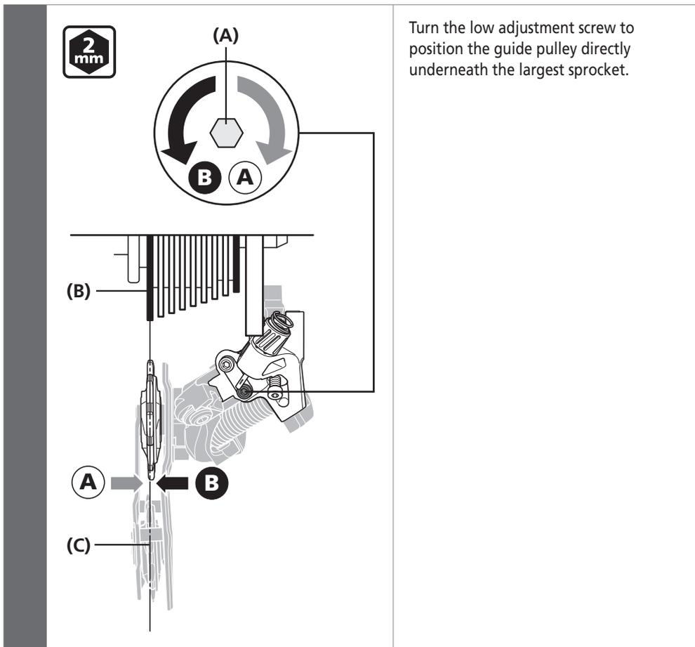
Turn the low adjustment screw to position the guide pulley directly underneath the largest sprocket.
