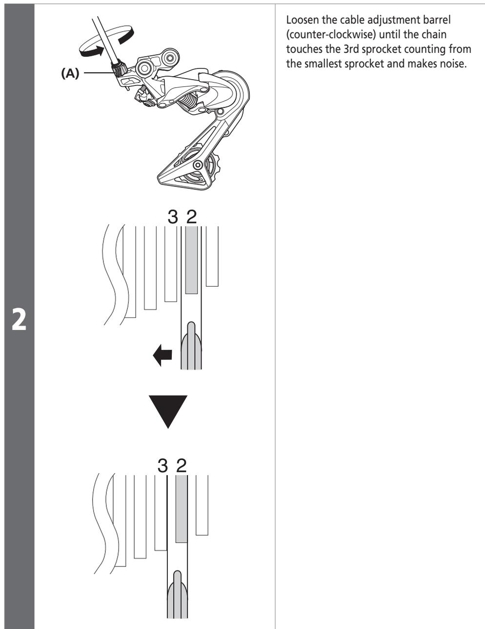
Loosen the cable adjustment barrel (counter-clockwise) until the chain touches the 3rd sprocket counting from the smallest sprocket and makes noise.
