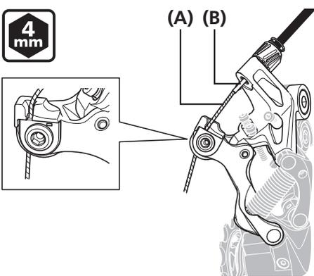
Connect the inner cable to the rear derailleur.
