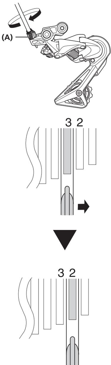
The diagram illustrates the adjustment process in three parts. At the top, a perspective view of the shift mechanism shows a cable adjustment barrel labeled (A) with a clockwise rotation arrow. Below this, a side-view diagram shows the chain on sprockets 3 and 2. An arrow points to the right, indicating the chain's position. A downward-pointing triangle indicates the next step. The final diagram shows the chain shifted back to sprocket 2, with sprockets 3 and 2 labeled above it.
