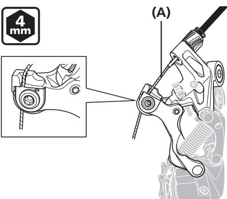
Reconnect the inner cable to the rear derailleur.
