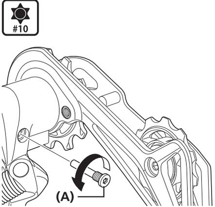
Using a Hexalobular[#10], remove the stopper bolt.
