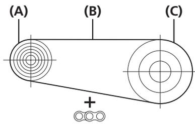
Mount the chain on to the largest sprocket and the largest chainring.
