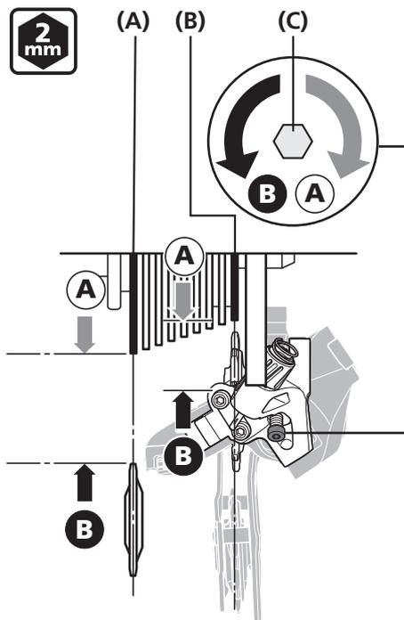
Mount the chain on the largest sprocket, and shift gears turning the crank arm.
