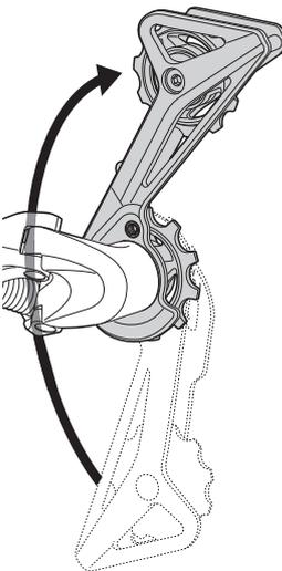
Turn the plate to loosen the plate tension spring as shown in the illustration.
