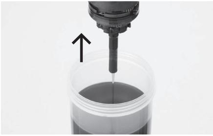
Remove the internal unit from the oil.
