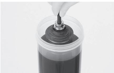
Keep the internal unit immersed for approximately 90 seconds.
