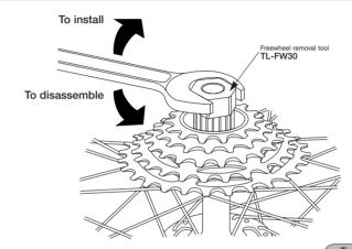
Tightening torque: 30 N⋅m {260 in. lbs.}
