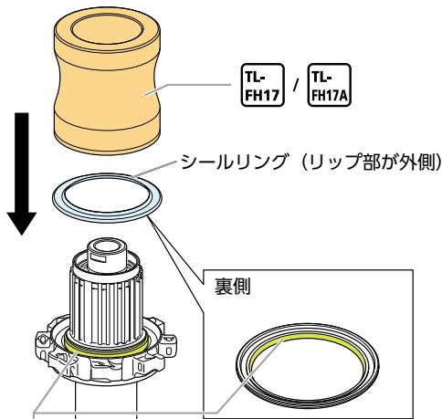
Seal Grease for Freehub (Y38Z98000)
