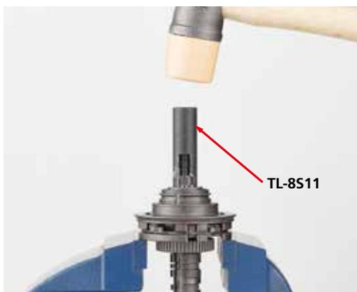
**13. Retirez le cône droit.**
