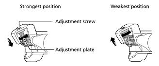
If the adjustment plate is at the strongest or the weakest position, do not turn the adjustment screw any further.
