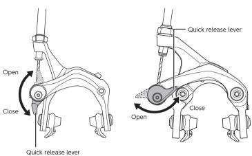
For models with a CLOSE position mark on the quick release lever and brake caliper side, align the marks. At this time, check for a click.
