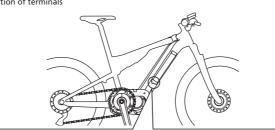
Battery (terminal) Battery mount (terminal)
