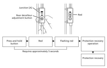
When the red LED of junction [A] is lit, the rear derailleur will not shift. Press the rear derailleur adjustment button until the red LED turns off.
