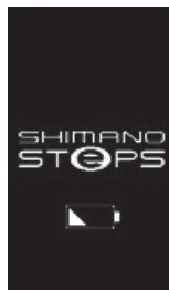
Battery level too low
