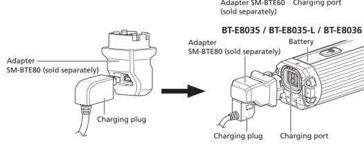
BT-E8010 / BT-E8014 / BT-E8016 / BT-E8020 1. Plug the charger's power plug into the outlet. 2. Plug the charging plug into the charging port.
