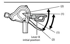
Gears can be shifted by pushing or pulling the lever. Some models have two-step gear shifting. Example: From the 4th to 3rd sprocket
