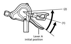
(1) Shifts one sprocket Example: From the 3rd to 4th sprocket
