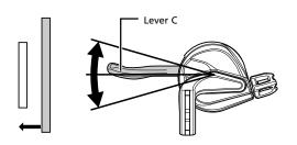
Gears can be shifted by pushing or pulling the lever.
