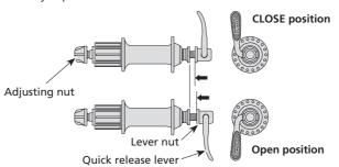
The clamping strength is adjusted by turning the adjusting nut. When the nut is turned in a clockwise direction, the clamping strength increases, and when the nut is turned in a counter-clockwise direction, the clamping strength decreases.
