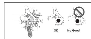
2. Open and close the guick release lever with your right hand while gradually tightening the adjusting nut with your left hand in the clockwise direction. Continue tightening the nut until you feel resistance with your hand at the point when the lever is parallel to the hub (as indicated by the dotted position in the diagram on the right).
