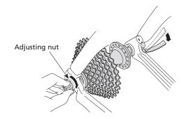
• If the clamping strength is adjusted too strong and the guick release lever cannot be pushed to the CLOSE position, turn the adjusting nut in a counter-clockwise direction to reduce the clamping strength. When doing this, do not fully release the adjuster nut. Turn it 1/8 of a revolution, and then try to push the lever to CLOSE, to set the maximum clamping strength with which you can push the quick release lever to the CLOSE position.
