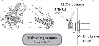
If there are any instructions on the tightening position for the E-THRU lever in the Service Instructions, follow them when tightening.
