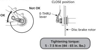
If there are any instructions on the tightening position for the E-THRU lever in the Service Instructions, follow them when tightening.
