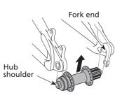
Move the E-THRU lever to the OPEN position, and insert it into the hole in the fork end on the side opposite to where the thread is. Pass the lever axle all the way through until it reaches the thread part on the other side.
