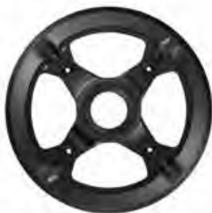
NEW SM-CRE80-12-SB Chainring for E-MTB (34T)
