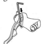
3. The return spring and cable hook can also be disassembled.
