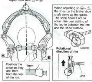
8. Fix by tightening the shoe fixing nut.
