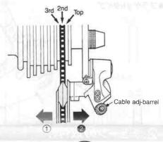
3. Next with the chain on the 2nd gear, increase the inner cable tension 1 while turning the crank forward. Stop turning the cable adjusting barrel just before the chain makes noise against the 3rd gear. This completes the adjustment
