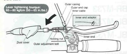
■The use of 2-mm inner cable and 6-mm outer casing is standard.
