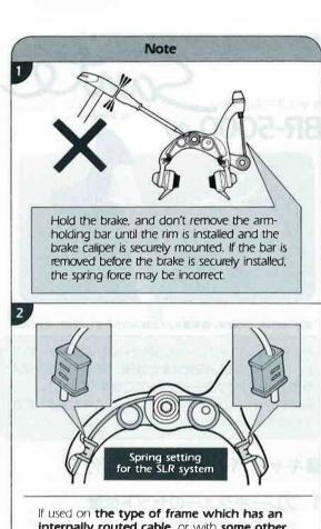
If used on the type of frame which has an internally routed cable, or with some other brake lever and outer cable, increase the return spring force as shown below.
