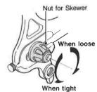
Cam lever tightening torque: 90-120 kgfcm (80-105 in.lbs.)
