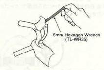
Clamp bolt tightening torque: 60-80 kgfcm (50-70 in.lbs.)
