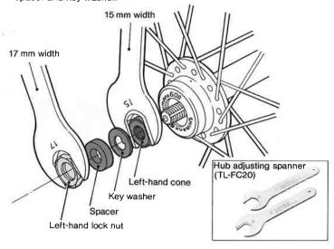
Next, pull the hub axle out to the right side. Remove the nine ball bearings on both right and left. Be careful not to remove the right and left dust caps at this time.
