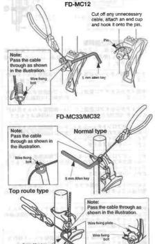
After taking up the initial slack in the cable, re-secure to the front derailleur as shown in the illustrati
