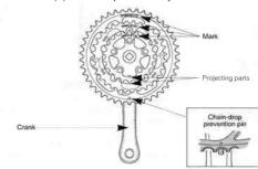
The features of the SIS will not be obtained if the chainrings are installed in the incorrect position, or if a chainring with a mark other than J- is being combined. Therefore, be sure to install them in the correct position.
