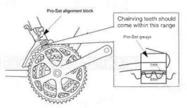
2. The level section of the chain guide outer plate should be directly above and parallel to the largest chainring.
