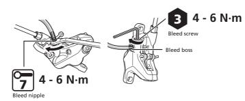
10. If the lever is slowly operated, air bubbles in the system will rise up into the oil funnel. Once the air bubbles stop appearing, depress the lever as far as it will go.
