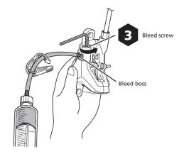
4. Once there are no more air bubbles mixed in with the oil, temporarily tighten the bleed nipple/bleed screw, and remove the syringe.
