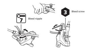
9. Repeat step 8 two to three times, then tighten the bleed screw/bleed nipple.
