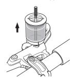
15. Tighten with a bleed screw to which an O-ring has been attached. Tighten until oil flows out to make sure that no air bubbles remain inside the reservoir tank. Do not operate the brake lever. If operated, there is a risk of air bubbles entering the cylinder. For information on the tool size and tightening torque for the bleed screw, refer to the dealer's manual for each model.
