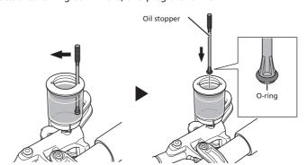
14. Remove the oil funnel with the oil stopper still in place.
