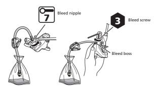
8. With the lever depressed, loosen and tighten the bleed screw/bleed nipple in rapid succession.
