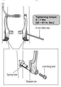
2. While holding the shoe against the rim, adjust the amount of shoe protrusion by changing over the washer B (thick or thin) so that dimension A is kept at 39 mm or more.
