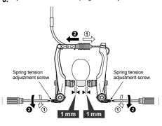
6. Depress the brake lever about 10 times as far as the grip and check that everything is operating correctly and that the shoe clearance is correct before using the brakes.
