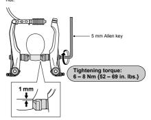
4. Pass the inner cable through the inner cable lead, and after setting so that the total of the clearances between the left an right shoes and the rim is 2 mm, tighten the cable fixing bolt.
