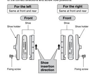
4 Tighten the fixing screw
