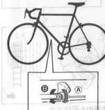
Cable adjusting barrel
