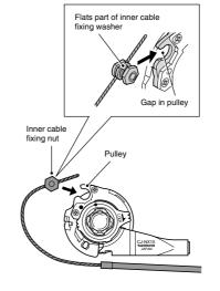
8. Turn the cable 60° counterclockwise and attach it
