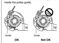
10. Secure the cable to the frame with the outer
