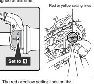
cassette joint are located in two places. Use the one that is easiest to see. When bicycle is standing up Should be straight When bicycle is upside down Should be straight
