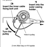
Note: Check that the inner cable is correctly seated inside the pulley guide
