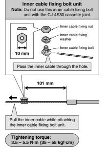
Bring the cable around to the cassette joint pulley, hold so that the inner cable fixing nut is facing to the outside (toward the fork end), and then slide the flats part of the inner cable fixing washer into the gap in the pulley.
