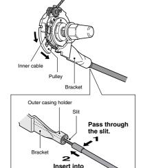
If first inserting the outer casing into the outer casing holder is easier, then first insert the outer casing into the outer casing holder and then insert a 2 mm Allen key or a #14 spoke into the hole in the cassette joint pulley, and then turn the pulley so that the inner cable fixing bolt unit fits into the gap in the pulley.
