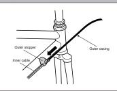
Confirm Make sure the outer casing is firmly seated in the outer stopper
