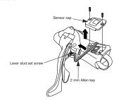
2. Insert a 2.5 mm Allen key or similar tool into the lever stud hole, and tap it gently with a plastic mallet to push out the lever stud. When the lever stud comes out, the bracket body and lever body can be disassembled. After this, pull the sensor cable out from the bracket
