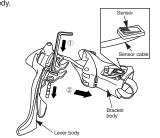
When removing the sensor cable, do not apply too much force when pulling the cable, otherwise the sensor may become damaged. Use a tool to hold the sensor in place and pull the cable out carefully.
