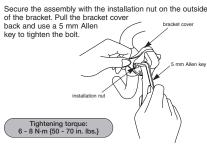
In the case of carbon handlebars, it may be necessary to lower the tightening torque in order to prevent damage to the handlebar. Please consult the bicycle or handleba manufacturer regarding the appropriate level of tightening torque for carbon handlebars.
