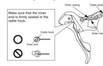
Bring the outer casing along the front of the handlebar and cover it with the outer guide. Now cut the outer guide to the length of the handlebar, and tape it temporarily in
