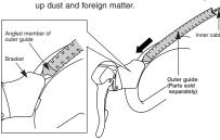
4. Set the outer casing on the inner cable, and in the bracket along the outer guide
