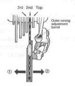
(2) Next with the chain on the 2nd gear, increase the inner cable tension ① while turning the crank arm forward. Stop turning the outer casing adjustment barrel just before the chain makes noise against the 3rd gear.
