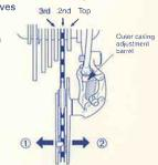
(2) Next with the chain on the 2nd gear, increase the inner cable tension ① while turning the crank arm forward. Stop turning the outer casing adjustment barrel just before the chain makes noise against the 3rd gear.
