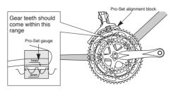
The level section of the chain guide outer plate should be directly above and parallel to the largest chainring.
