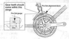
The level section of the chain guide outer plate should be directly above and parallel to the largest chainring. Secure using a 5mm Allen key.
