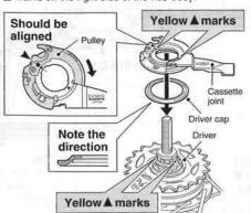
2. Secure the cassette joint to the hub with the snap ring. Insert the snap ring securely into the groove of the right hand lock nut at this time,
