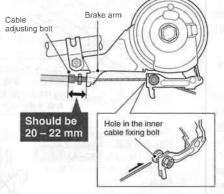
2. Check that both ends of the outer casing are securely inserted into the cable adjusting bolts of both the
