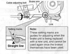
After depressing the brake lever to check the braking performance, secure the cable adjusting bolt with the cable adjusting nut.
