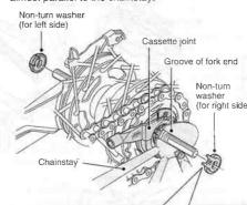
Different types of left and right non-turn washers are provided for use with standard and reversed fork ends. Use whichever nonturn washers are suitable
