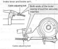
3. Pull the link back until it stops. Then, while pulling the inner cable to apply the full amount of tension to the cable, tighten the inner cable fixing nut.
