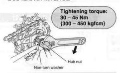
When installing a part such as a mudguard stay to the hub axle, install in the order shown in the illustration below.
