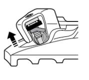
If the adjustment plate is at the strongest or the weakest position, do not turn the adjustment bolt any further.
