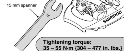
Tightening torque: 35 – 55 N·m {304 – 477 in. lbs.}
