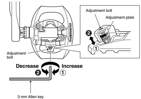
When the adjustment bolt is turned clockwise, the spring tension increases, and when it is turned counterclockwise, the spring tension decreases.
