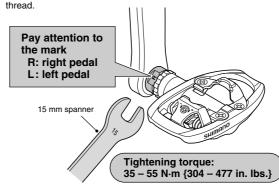
A 6 mm Allen key cannot provide a sufficient tightening torque. Always be sure to use a 15 mm spanner
