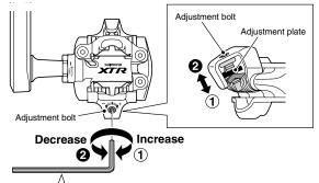
PD-M970: 2.5 mm Allen key PD-M770/PD-M540/PD-M530/PD-M520: 3 mm Allen key
