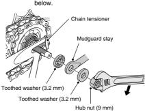
Tightening torque: 30 – 45 N·m {300 – 450 kgf·cm}
