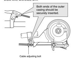
Pull the link back until it stops. Then, while pulling the inner cable to apply the full amount of tension to the cable, tighten the inner cable fixing nut.
