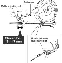
Check that both ends of the outer casing are securely inserted into the cable adjusting bolts of both the brake lever and brake arm.
