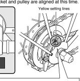
The yellow setting lines on the cassette joint are located in two places. Use the one that is easiest
