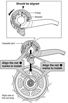
Secure the cassette joint to the hub with the cassette joint fixing ring. When installing the cassette joint fixing ring, align the yellow
