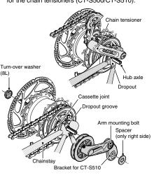
Place the non-turn washers on the right side and left side of the hub axle. At this time, turn the cassette joint so that the projecting parts of the non-turn washers fit into the grooves of the dropouts and the cassette joint follows the inside of the chainstay
