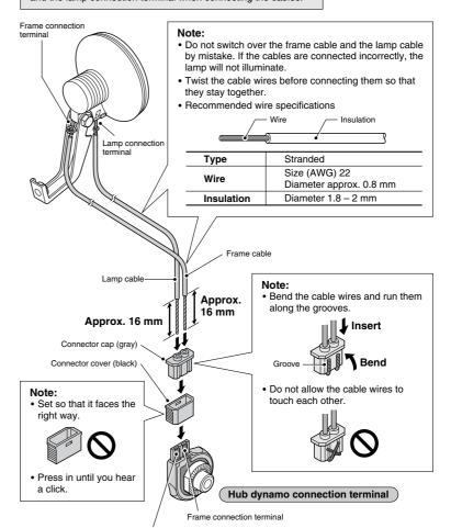
· Secure the cable to the front fork or the basket stay so that it will not get caught in the spokes or any other parts while riding. If the position of the hub dynamo may change with respect to the lamp while riding, for example when using a suspension fork, make sure that the cable is connected so that it will not be too loose or too tight at any point within the range of movement.
