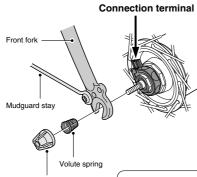
The toothed axle washer is not necessary for a quick release type.
